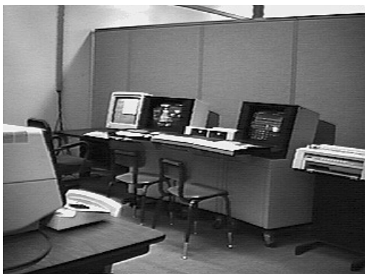
Fig. 2. Universal Station nodes forming part of the Honeywell TDC3000 system at ASU's Control Systems Engineering Laboratory
