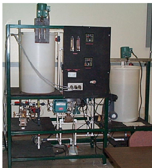
Fig. 1. Brine-water mixing tank schematic (top) and photograph (bottom).
