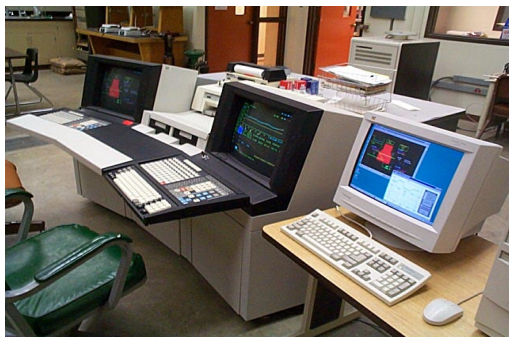
Fig. 3. Representative cluster of Universal and Global User Stations for ASU's TotalPlant Solution System.
